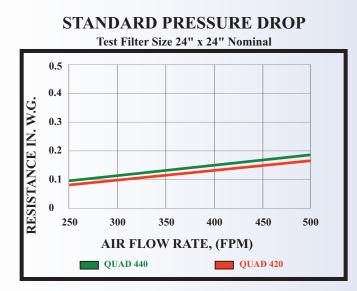
STANDARD PRESSURE DROP Test Filter Size 24" x 24" Nominal
