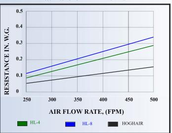
STANDARD PRESSURE DROP Test Filter Size 24" x 24" Nominal
